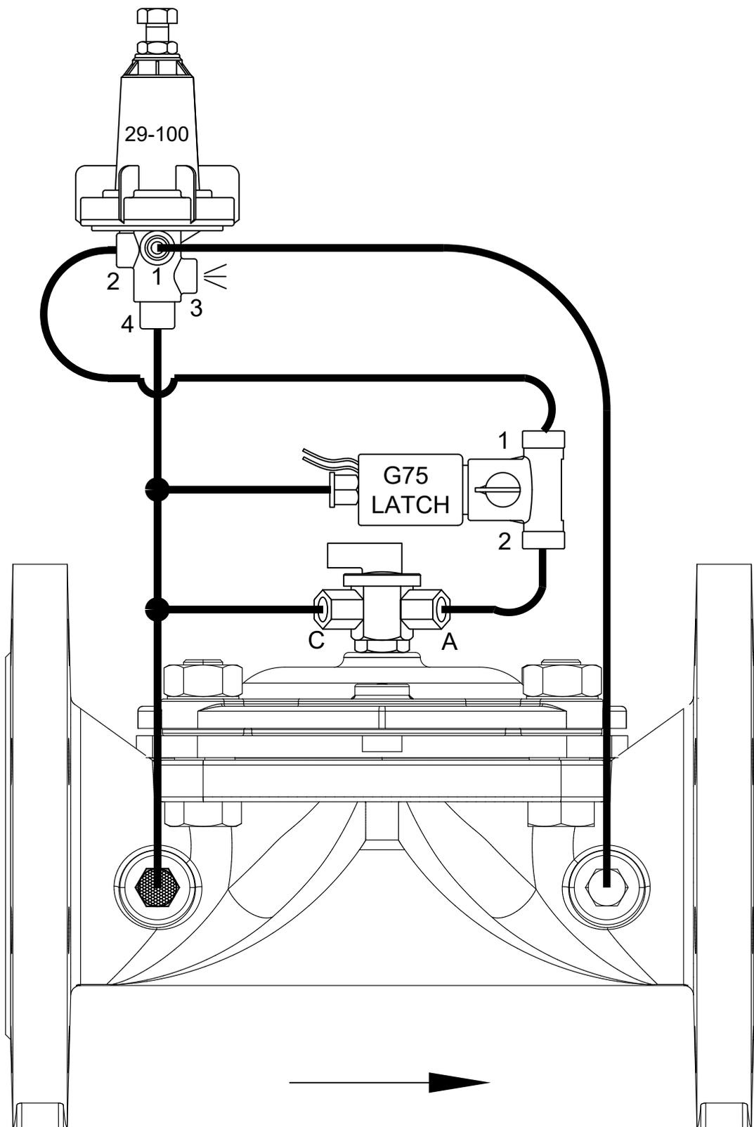
NOTE : NO ELECTRICAL COMMAND - VALVE IS CLOSED
