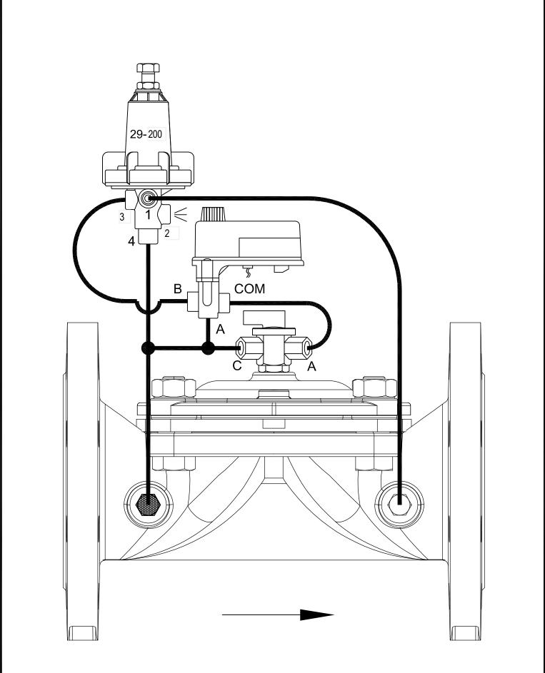
NOTE: NO ELECTRICAL COMMAND - VALVE IS CLOSED
