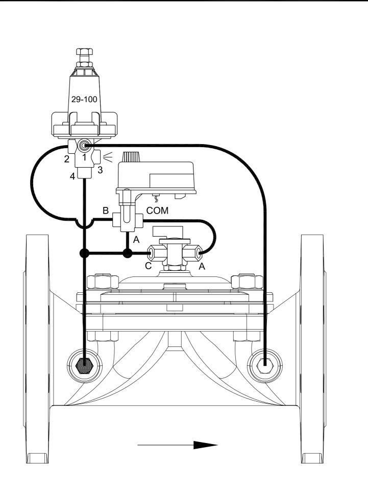
NOTE: NO ELECTRICAL COMMAND - VALVE IS CLOSED
