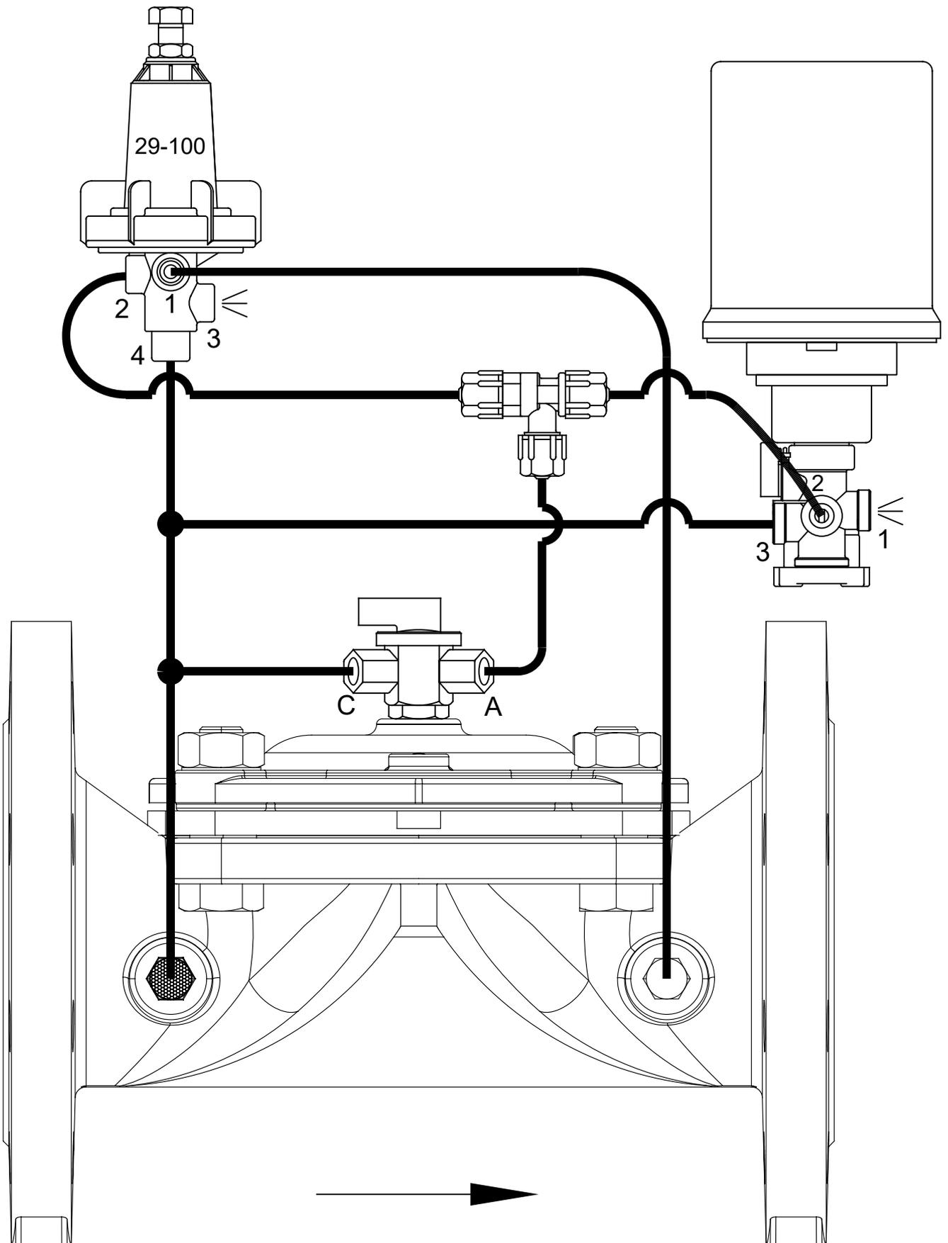
NOTE : NO ELECTRICAL COMMAND - VALVE IS CLOSED
