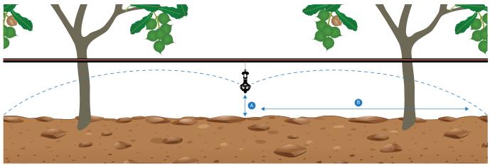
Due to the Flat Trajectory of the Sprinkler, there is minimal impact to Tree Foliage
