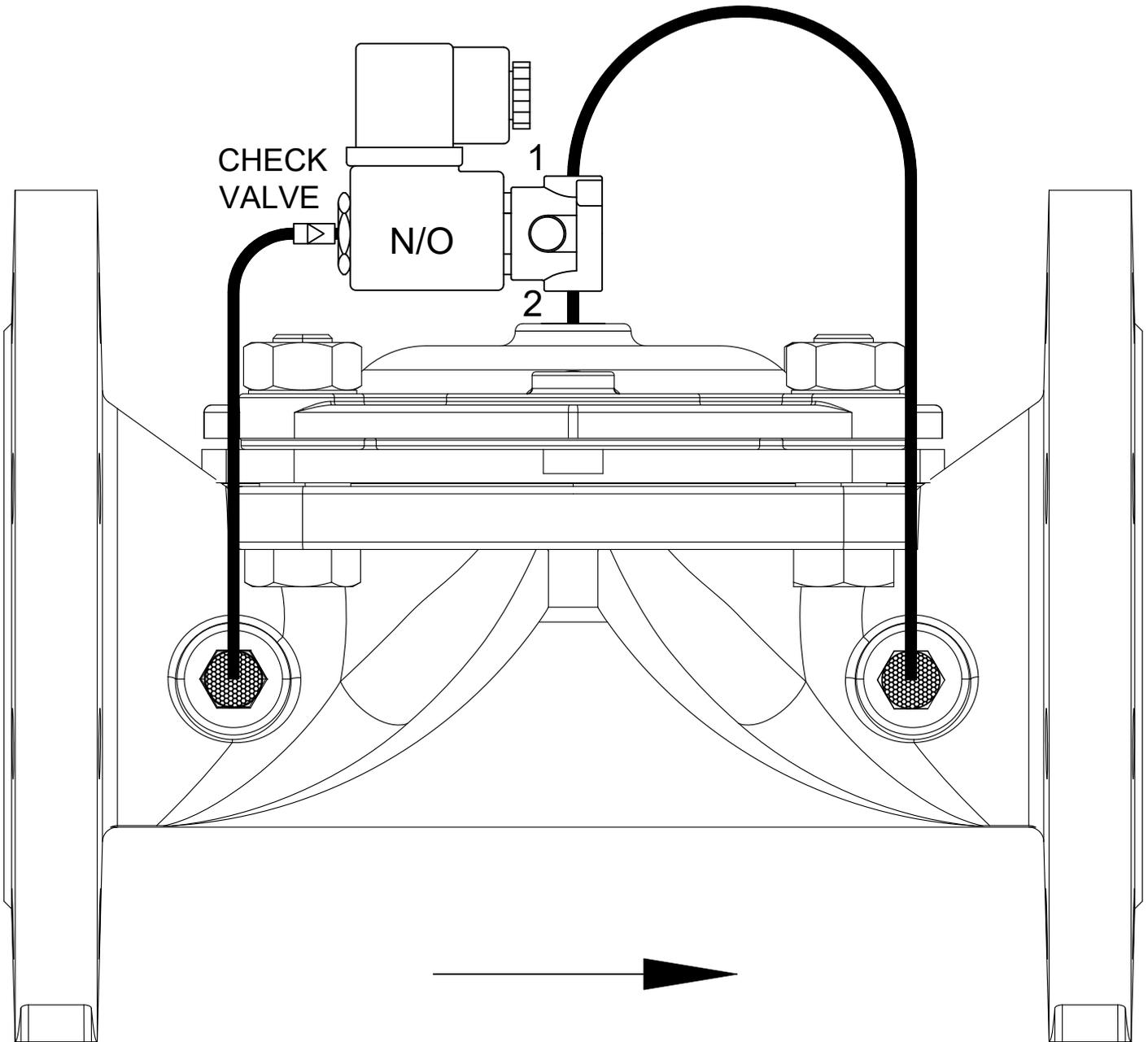
NO ELECTRICAL COMMAND - VALVE CLOSED
