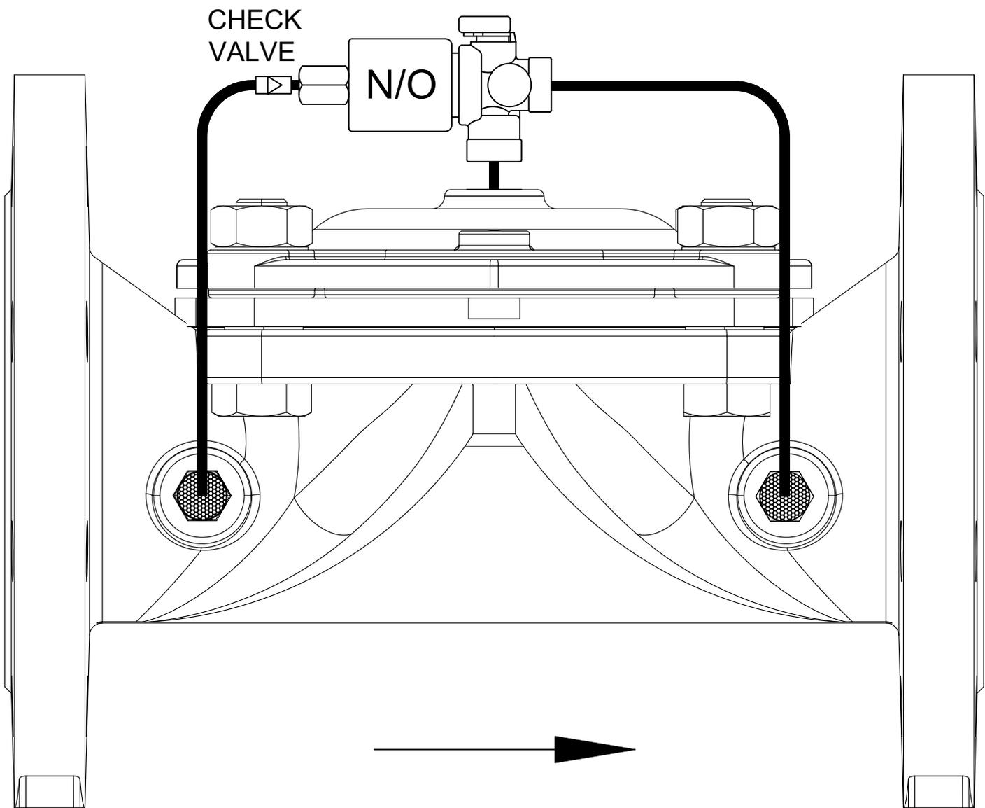
NO ELECTRICAL COMMAND - VALVE CLOSED
