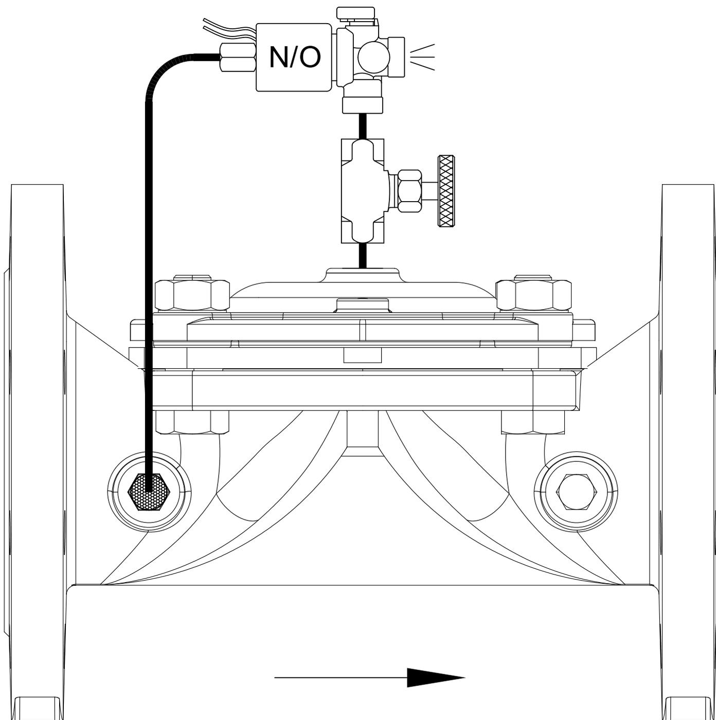
NO ELECTRICAL COMMAND - VALVE CLOSED
