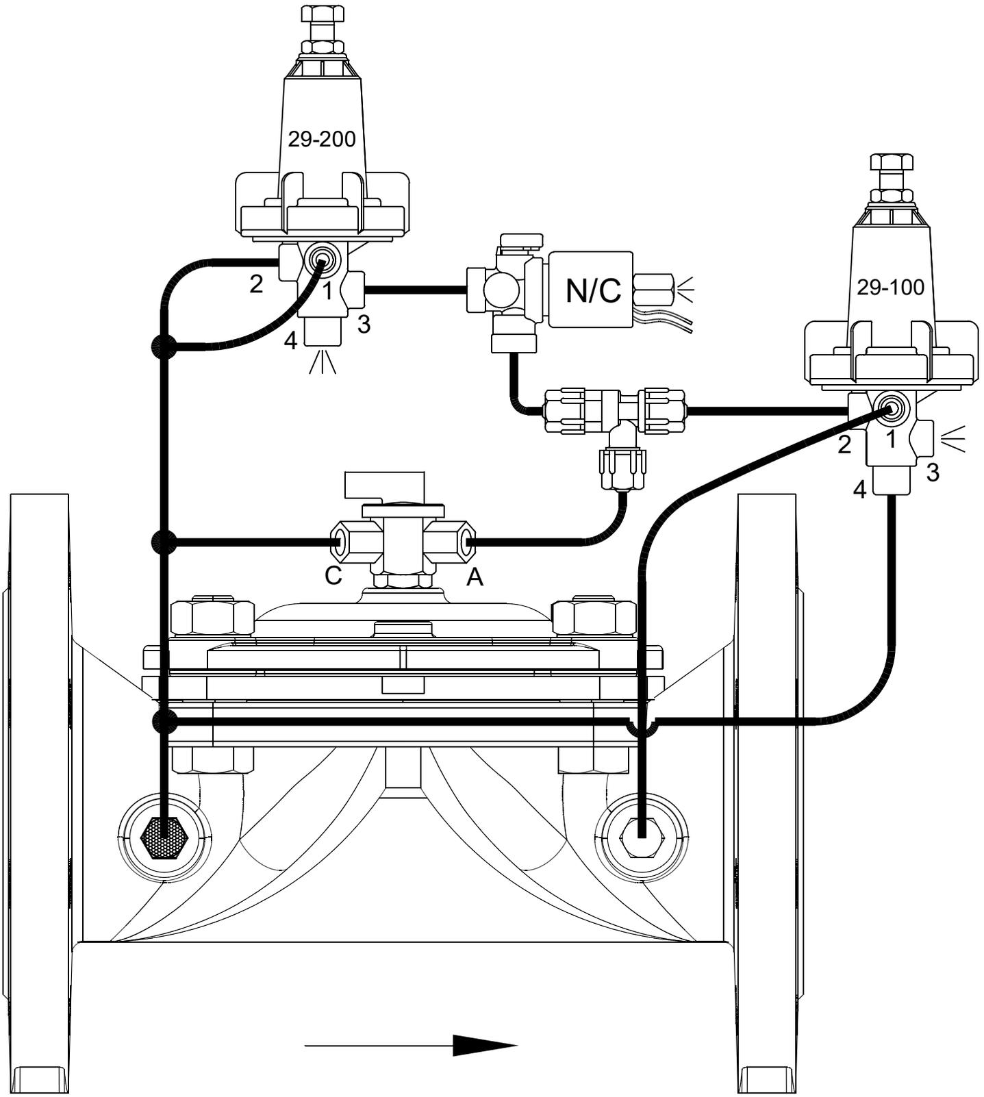
NOTE : NO ELECTRICAL COMMAND - VALVE IS HPR
