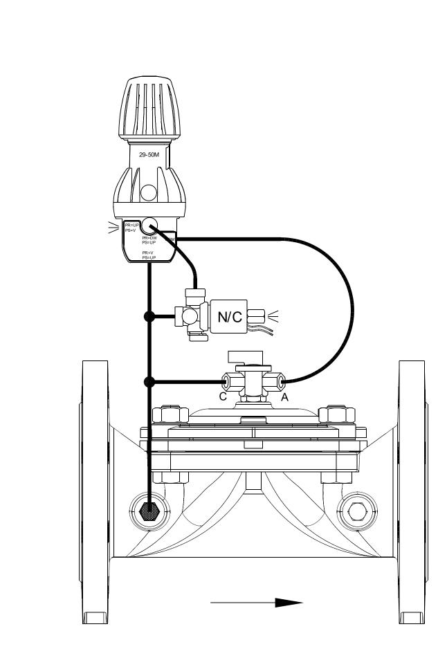
NOTE: NO ELECTRICAL COMMAND - VALVE IS CLOSED
