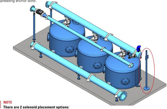
A. All the solenoids are placed on the solenoid bracket on the controller stand.
