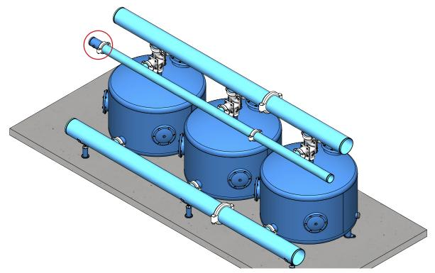
**b.** Connect the backwash flow-control value to the backwash manifold's short section with a grooved coupling. Be sure that the position of the value is per the flow arrow marked on the value.
