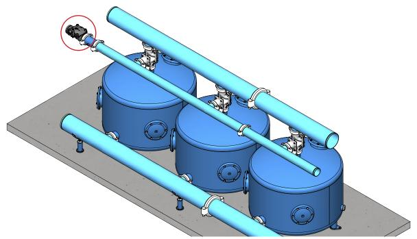
**c.** Connect the valve-command water-supply assembly to the dedicated outlet of the backwash manifold short section.
