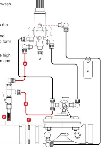
8. Connect the end-cap to the backwash manifold with a grooved coupling.
