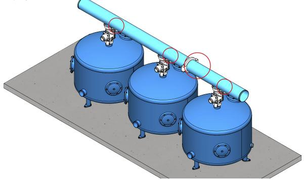
Connect the backwash manifold to the backwash valves and the backwash manifold sections to each other with grooved couplings.
