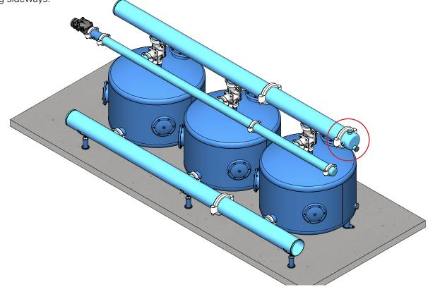
**10.** Connect the end-cap to the outlet manifold with a grooved coupling. Make sure that the end-cap is placed with the 1" outlet pointing upwards.
